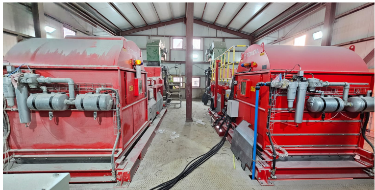
Fig.1 - XRT Sorting Plant fully commissioned; 2x Tomra XRT Sorters (COM Tertiary XRT 1200)
