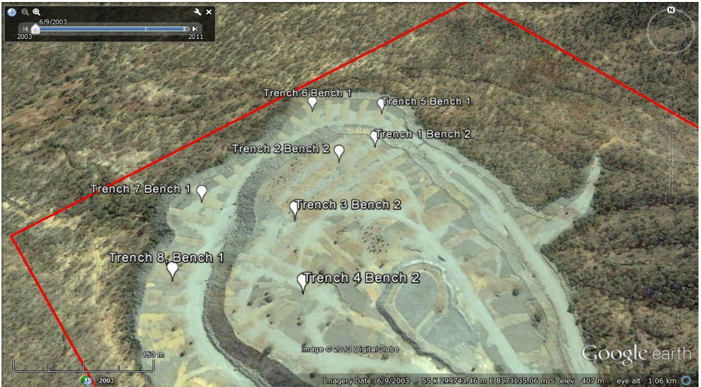
Figure 1. Locations of costeans excavated for bulk sample of stockpile for X-ray ore sorter trials and determination of global average grade.
