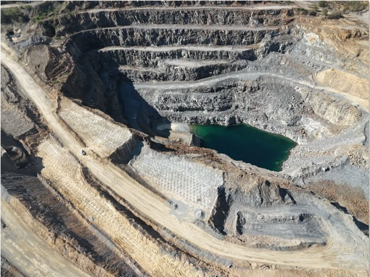
Picture above: Stripping ongoing in the South part of the pit to access the Iolanthe vein system, main ore body targeted in the Stage II Open Pit.
