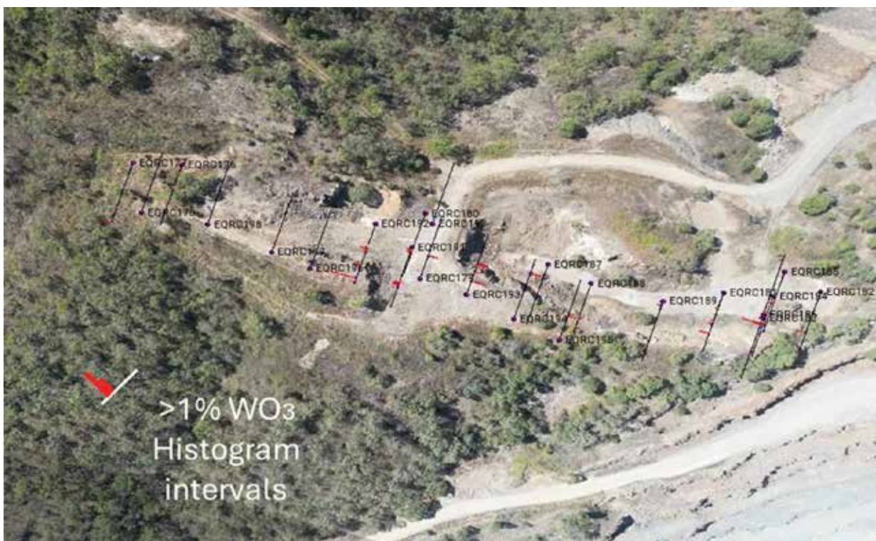
Ruby Vein section & plan showing thin veins at high level in the system. Shallow 50-meter holes hit 12 meters of grades up to 1.2% WO_3 .
