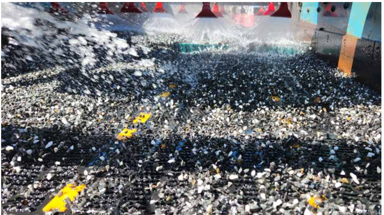
Fine ore being screened in a vibrating screen with new self-cleaning panels, ahead of the Mineral Jig at the Gravity Plant.
