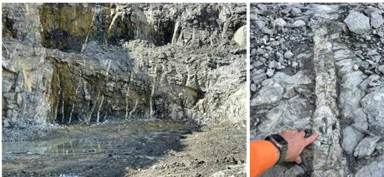
Level 295m RL confirms the thickening of the veins as seen on the cliff face looking into the Johnson Vein system.
