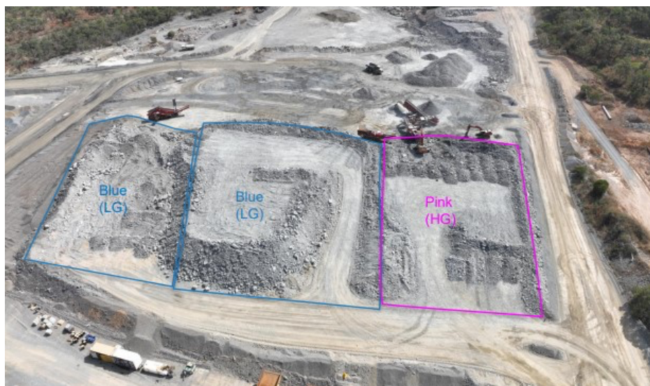
Picture Above: ROM 1 showing the separation of Low-Grade Ore (Blue: WO_3 0.08-0.2%) and High-Grade Ore (Pink: WO_3 > 0.2\% ).
