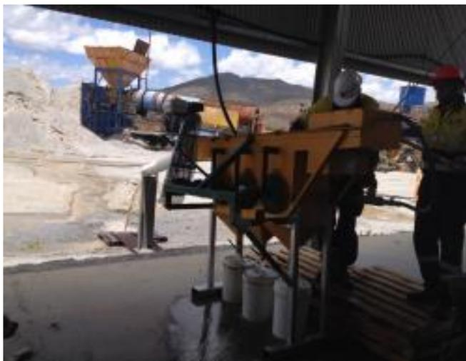
Jig Test Work – Tailings Retreatment Operation
