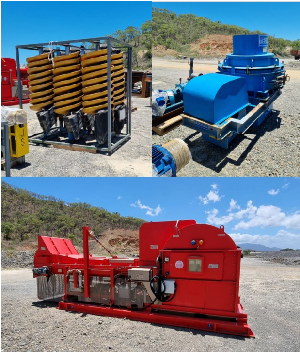
Fig.2 – Selected Early Works upgrades, covering a spirals circuit (top left), a vertical shaft impact crusher (top right) and an additional XRT Sorter (bottom).
