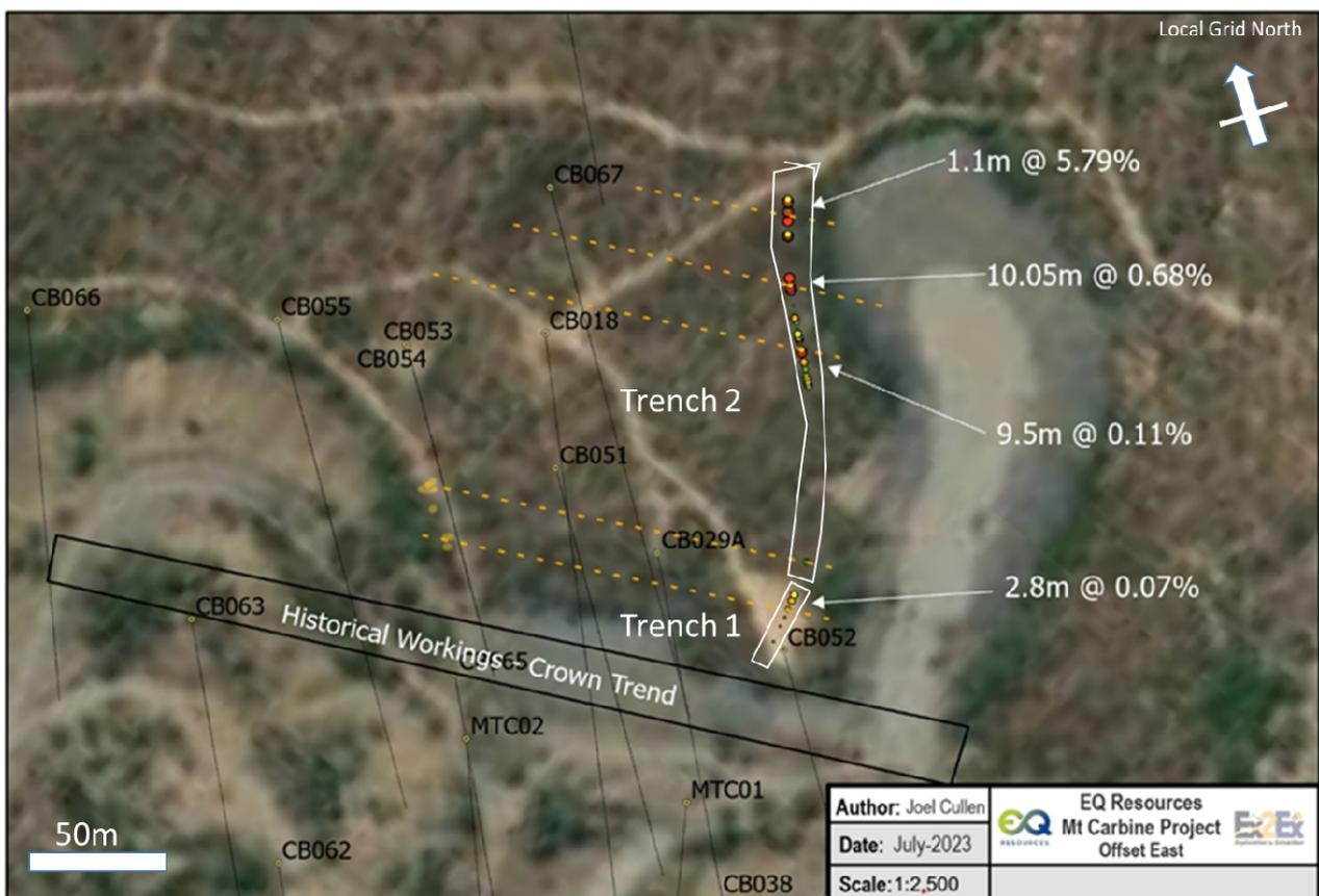
Fig.2 - Location of the two trenches and summary of results (grade shown in % WO<sub>3</sub>)
