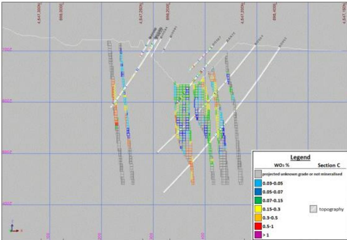
Figure 14-27 Section C (incl. drill hole BD052)
