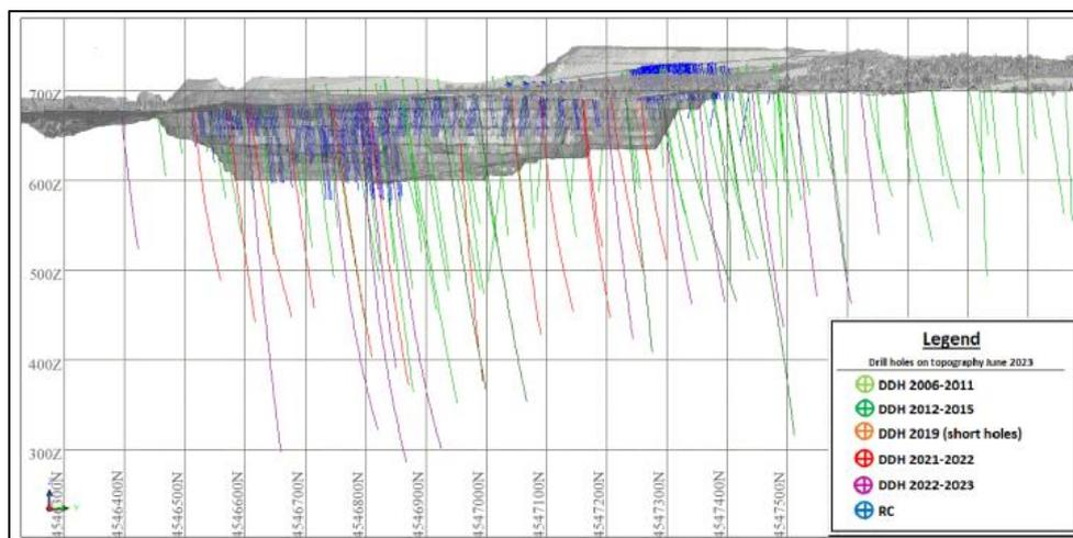
Fig. 2 - Long section of the deposit (North on left) showing topography, the pit and drill holes.
