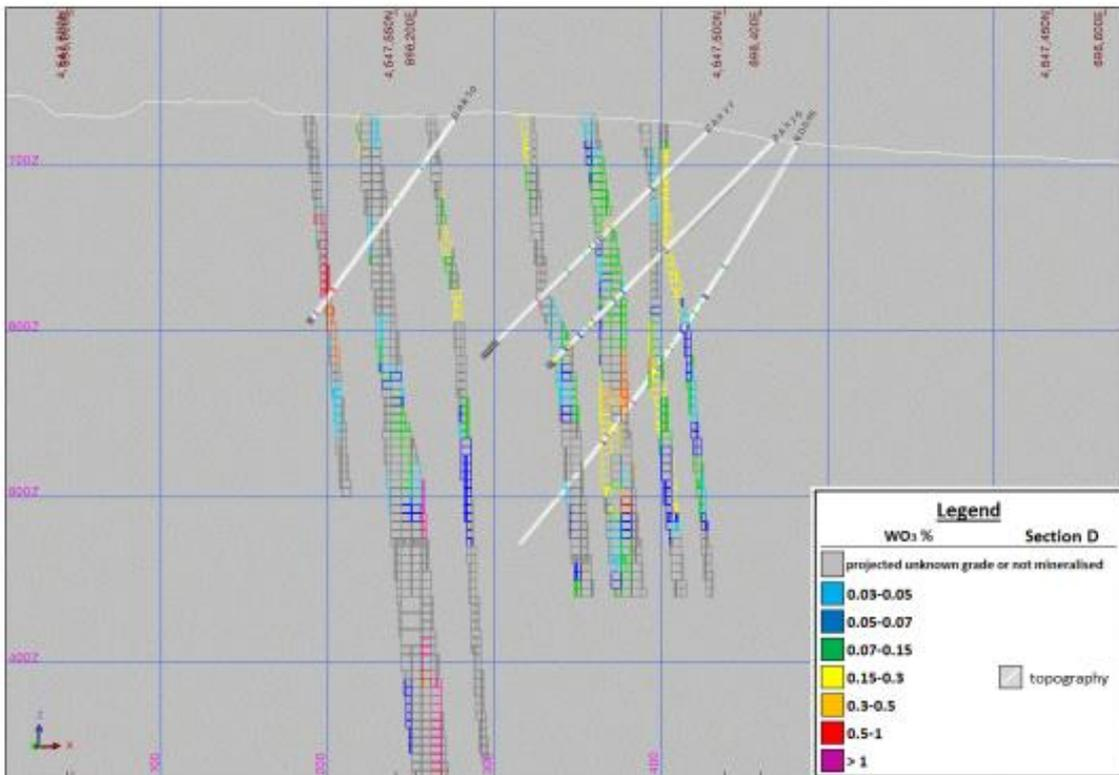
Figure 14-28 Section D (incl. drill hole BD045)
