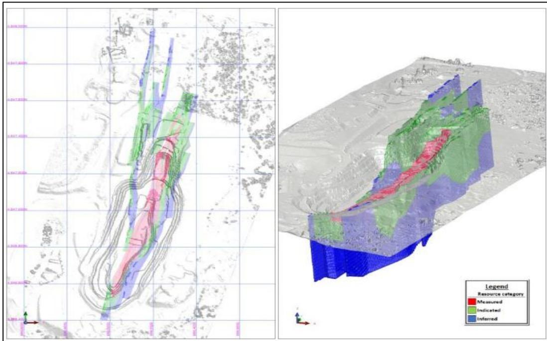
Fig. 4 - Plans and Isometrics showing the resource categories of the deposit and their location.
