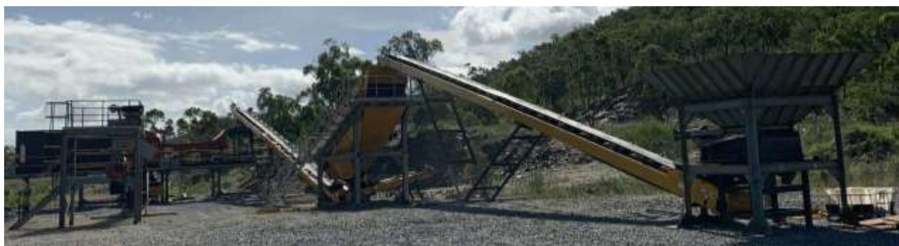
*Figure 3: Sensor Based Sorting (XRT Pilot Plant)*
