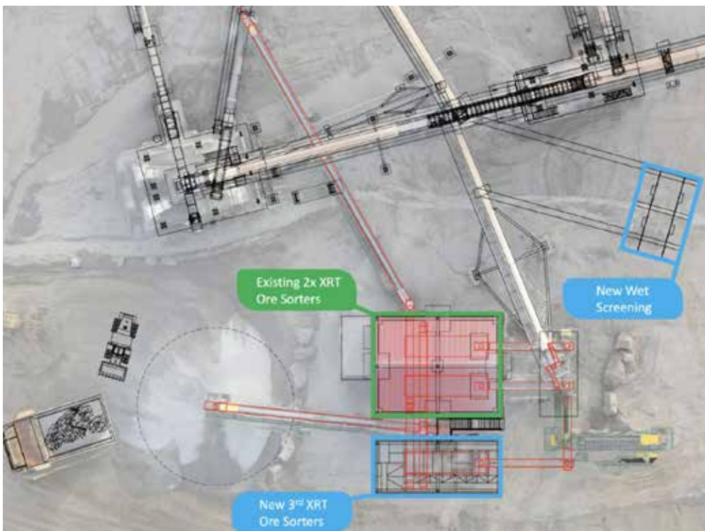
Figure above: Design sketch of the 3rd XRT Ore Sorter hangar and new wet screening station.
