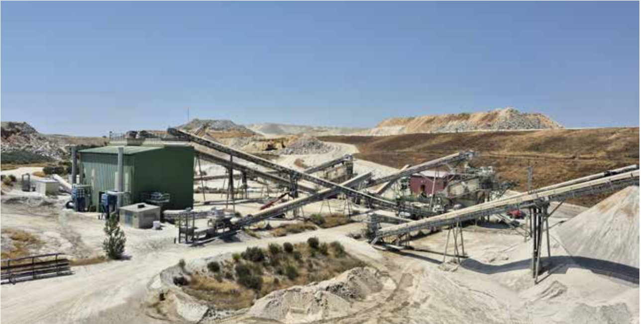
Picture above: Saloro's Processing plant with the Gravity Plant on the left and the Ore Sorter Plant in red in the background on the right.
