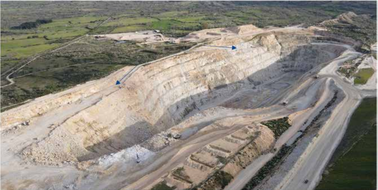
Picture above: The Eastern pit slope of the Barruecopardo Open Pit, blue arrows showing the ramps in Phase 7.
