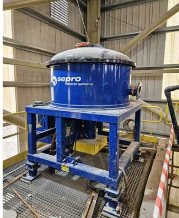
Picture above: The Falcon Concentrator prior to installation.
