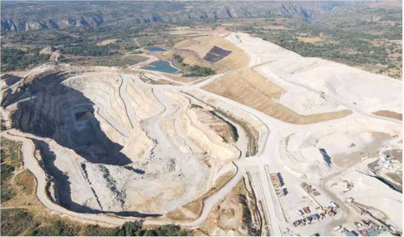
Picture above: Northern area of Phase 6 at elevation 700RL, including the access ramp and 690RL bench, with ore stockpile and waste dump as of the end of June 2025.
