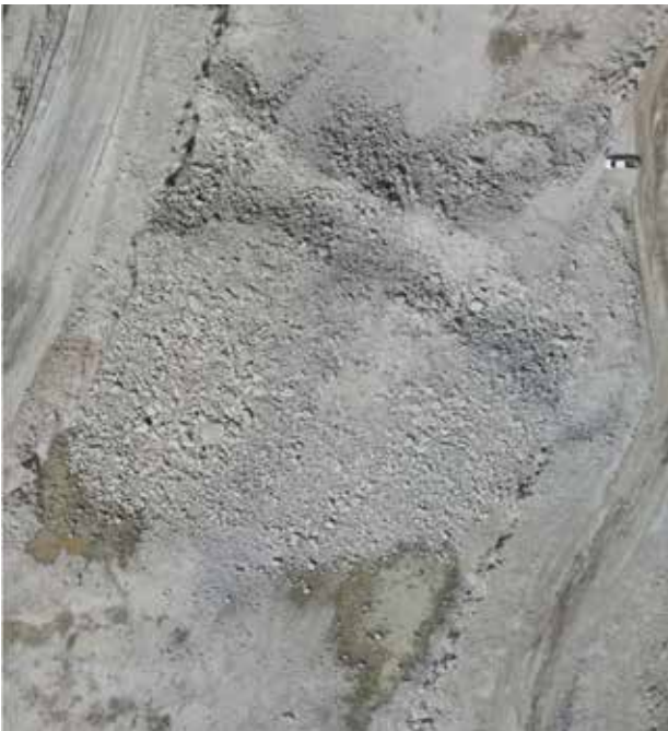
Pictured left: Result of blast 019_580F5M on a 10-metre bench. Pictured right: Simulation performed with the OREPRO 3D software before blasting showing how the mineral will be arranged for loading.
