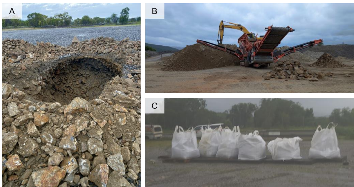
Figure 3: Site based pit sampling and screening. A) Initial sampling of Pit 5; B) Screening of bulk sample materials; C) Bulka bags of sub-sampled material from Pits 1 to 6 prior to dispatch to SMI.
