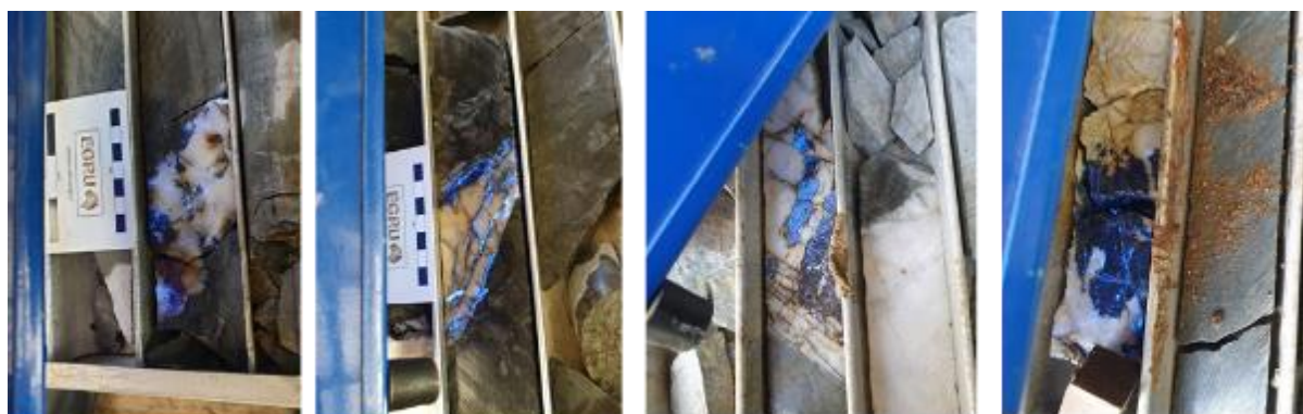
Figure 4-9: Late Replacement of Coarse wolframite by Fine Scheelite
