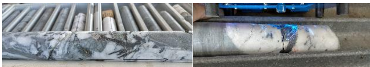
Figure 6-3: Examples of Coarse Wolframite with Scheelite Quartz
