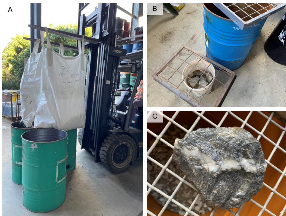
Figure 4: Screening of bulka bag samples from Pits 1 to 6 at the SMI – UQ Indooroopilly Pilot Plant. A) Transfer of samples from bulka bags to drums; B) Screening of bulk sample materials using Gilson screens; C) Example of +75 mm particle with quartz-wolframite-scheelite vein on Gilson screen.
