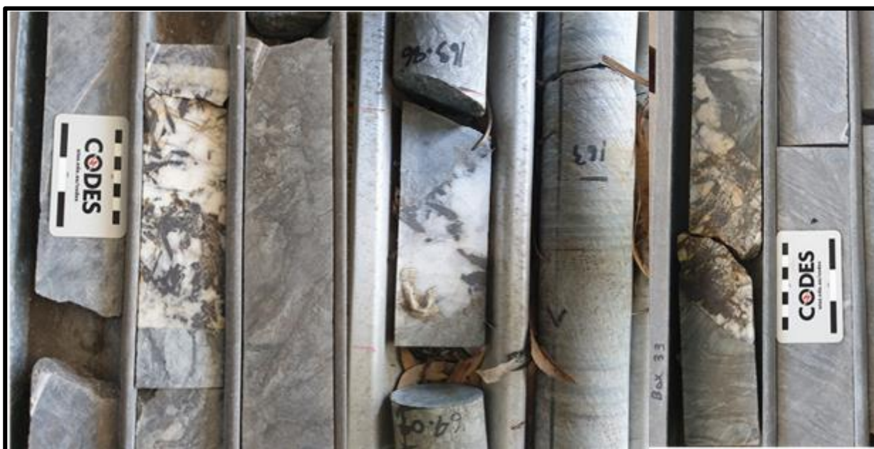
Figure 7: King Veins Showing Coarse Vein Textures of Wolframite Crystals
