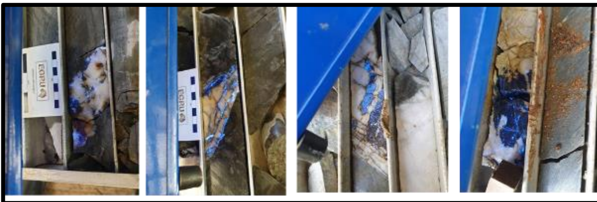
Figure 8: Core Showing Late Replacement of Wolframite by Fine Network Retrograde Scheelite
