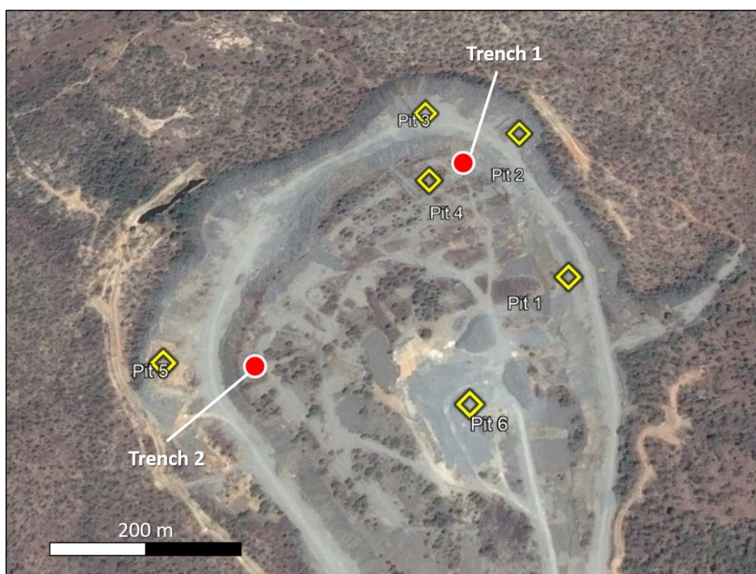
Figure 2: Location of trench samples 1 and 2 for the sorter trial and Pits 1 to 6 for the grade by size assessment within the low grade stockpile at Mt Carbine.
