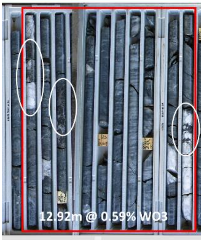
Figure 12: Zone of Silicified Cherts & Metasediments with King Veins on Margins
